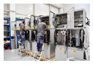
HELB participated in the supply and delivery of ZX0.2 MV substations for a wind farm connection substation in Bosnia and Herzegovina. This compact gas-insulated switchgear (GIS), manufactured by ABB, is characterized by high reliability, safety, and easy maintenance. Its modular design allows for quick installation and adaptation to specific user needs, making it an ideal solution for power distribution, industrial plants, and infrastructure
